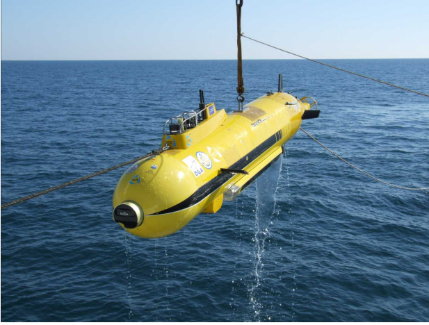
Fig. 5. Daurade : the underwater robot used for the experiment. The portside lateral sonar antenna corresponds to the one meter black segment at the bottom left of the robot
