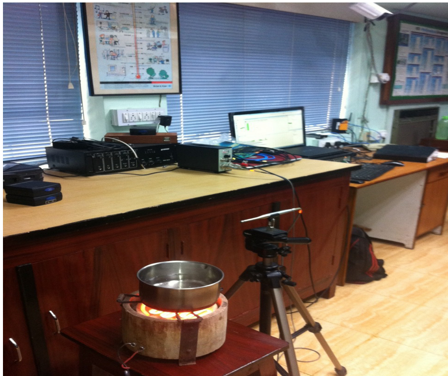
Figure 2: Boiling Experiment Set-up
