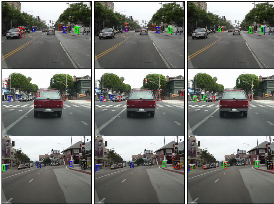
Fig. 6: Comparison of pedestrian detectors. From left to right, HOG, ChnFtrs and SmallPedCNN-merged detections. All detectors are setup to have a 1 FPPI rate on the far subset of the dataset. Green, blue and red boxes correspond respectively to Detections, Misses and False Positives. Solid lines correspond to ground truths and dotted lines to detections.
