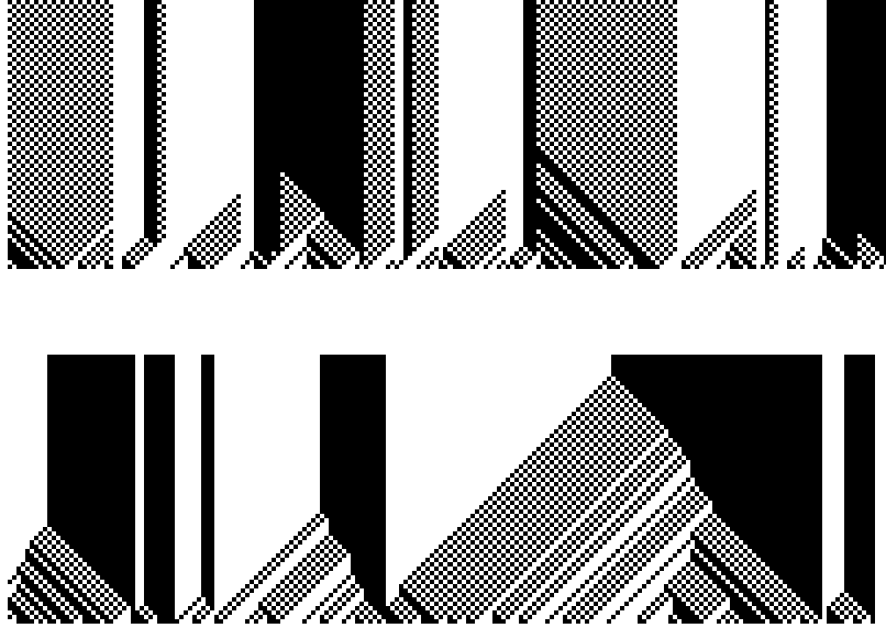
Figure 4: Example of dynamics for automata with rules in \{f, g, h\} . The automaton at the top is number conserving, while the one at the bottom is not. Time goes upward.
