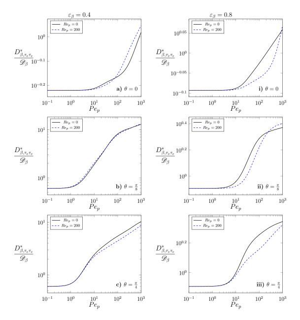
Figure 6: Transverse component of the total dispersion tensor vs.  $Pe_p$  taking three different values of  $\theta$ . Results are obtained from solving the associated closure problems in a 2D unit cell having porosities of 0.4 and 0.8 with the solid phase modeled as a square. Black curves correspond to  $Re_p = 0$  and blue curves correspond to  $Re_p = 200$ .
