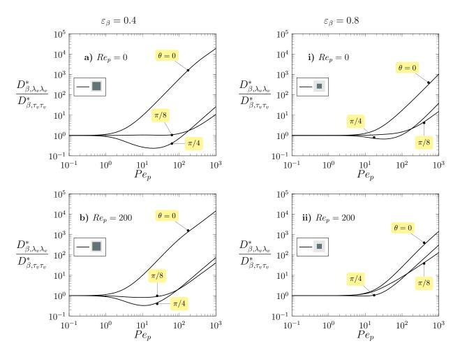
Figure 7: Dependence of the ratio of the longitudinal and transverse components of the total dispersion tensor with  $Pe_p$  for three flow orientations taking  $\varepsilon_{\beta} = 0.4$  and  $\varepsilon_{\beta} = 0.8$ . The results were obtained from solving the closure problems in unit cells with the solid phase represented by a square obstacle.
