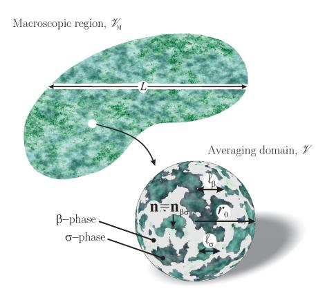
Figure 1: Sketch of the system, including characteristic lengths and a sample of the averaging domain.
