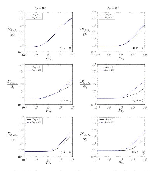
Figure 5: Longitudinal component of the total dispersion tensor vs.  $Pe_p$  taking three different values of  $\theta$ . Results are obtained from solving the associated closure problems in a 2D unit cell having porosities of 0.4 and 0.8 with the solid phase modeled as a square. Black curves correspond to  $Re_p = 0$  and blue curves correspond to  $Re_p = 200$ .
