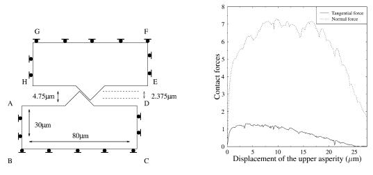
Figure 12. Asperity shearing—geometry.
