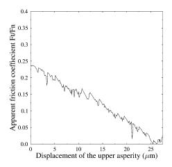
Figure 14. Asperity shearing-friction coefficient.
