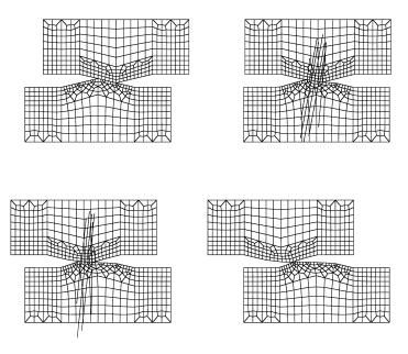
Figure 15. Asperity shearing-deformed mesh.
