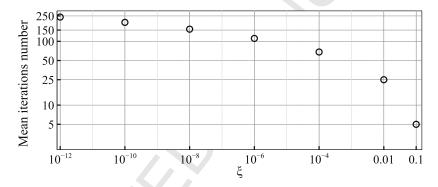
Figure 7: Mean number of iterations performed to reach the specified tolerance  $\xi$  for the heptane/air autoignition test case when methods I and III are chosen to solve the variable-coefficient Poisson Eq. (63).
