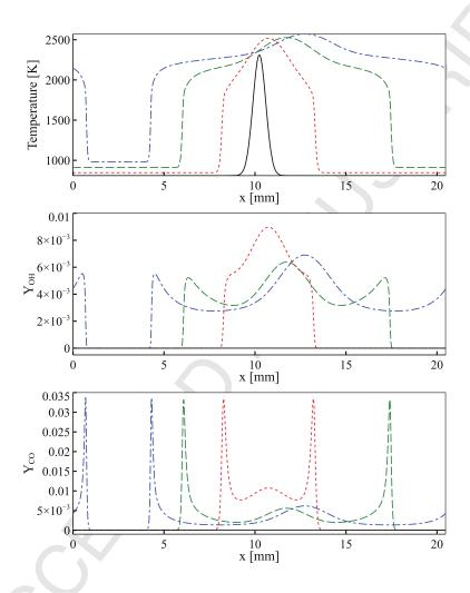
Figure 2: Structure of a freely propagating one-dimensional premixed methane/air flame in a closed domain at 101325 Pa and equivalence ratio of  $\Phi=0.6$ . Top: temperature. Middle:  $Y_{\rm OH}$ . Bottom:  $Y_{\rm CO}$ . Solid line ( ——— ) initial solution at t=0 ms. Dotted line ( ——— ): t=1.50 ms. Dashed-dotted line ( ——— ): t=2.50 ms.
