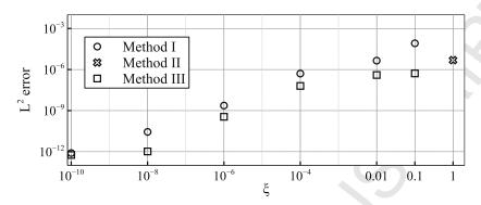
Figure 8:  $\mathcal{L}^2$  norm errors of the velocity field at t=1 ms formed by methods **I**, **II** and **III** respect to the tolerance parameter  $\xi$  for the 2D Vortex-Flame test case.
