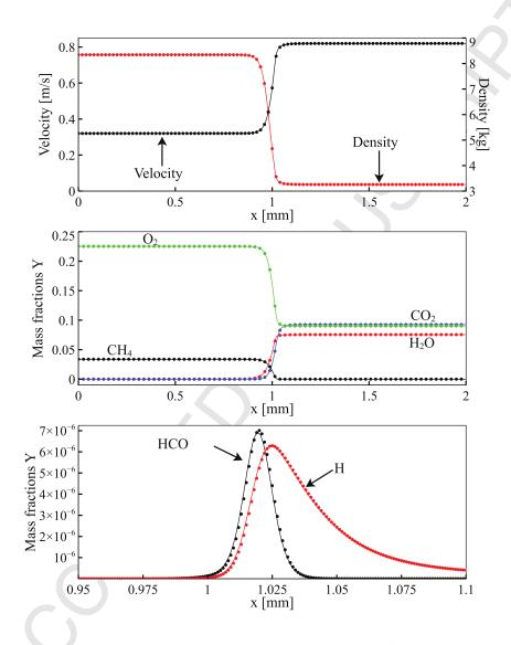
Figure 1: Structure of a steady one-dimensional premixed methane/air flame at  $2 \times 10^6$  Pa and equivalence ratio of  $\Phi = 0.6$ . Solid line ( ——): initial solution interpolated from a **CHEMKIN** simulation. Symbols (•): solution  $S_{init}$  computed at 1 ms with **HOLOMAC** on a fine mesh ( $\Delta x = 1 \ \mu m$ ) and a very small time-step ( $\Delta t = 1 \times 10^{-8}$  s).
