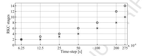
Figure 9: Minimum number of iterations of the RKC method to ensure stability for different values of  $\Delta t$  ranging from  $6.25 \times 10^{-8}$  s to  $2.75 \times 10^{-6}$  s. The configuration investigated is the freely propagating 1D premixed methane flame in a closed, periodic domain (see §4.1.2). Circle symbol ( $\bigcirc$ ): number of stages K. Cross symbol ( $\times$ ): number of stages L.
