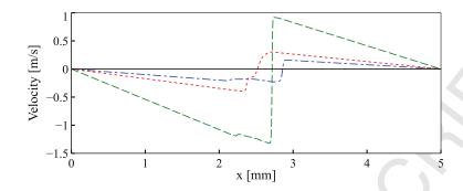
Figure 5: Velocity of the flow during an autoignition sequence of a one-dimensional flame into mixing layers of heptane and air, at  $4 \times 10^6$  Pa. Solid line ( —— ) initial solution at t=0 ms. Dotted line ( —— ): t=0.1 ms. Dashed line ( ——— ): t=0.2 ms. Dashed-dotted line ( ——— ): t=0.3 ms.
