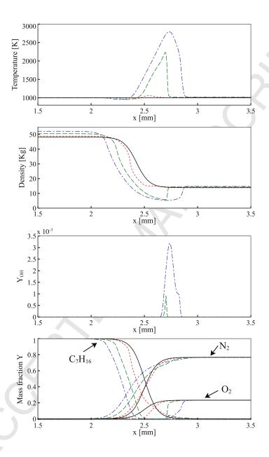
Figure 4: Structure of an autoignition sequence of a one-dimensional flame into mixing layers of heptane and air, at  $4 \times 10^6$  Pa. Solid line ( — ) initial solution at t = 0 ms. Dotted line ( — ): t = 0.1 ms. Dashed line ( — — ): t = 0.2 ms. Dashed-dotted line ( — — ): t = 0.3 ms.
