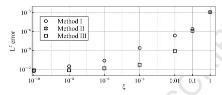
Figure 6:  $\mathcal{L}^2$  norm errors of the velocity field at t=3 ms formed by methods **I**, **II** and **III** respect to the tolerance parameter  $\xi$  for the heptane/air autoignition test case.
