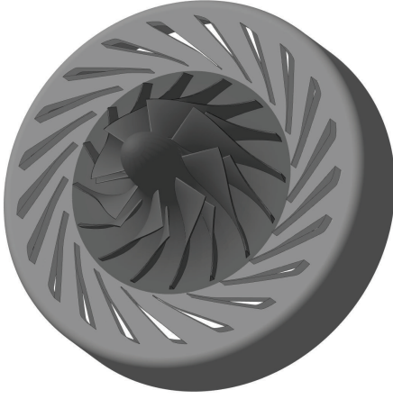
FIGURE 1: 3D sketch of the compressor stage hub with the return downstream channel.
