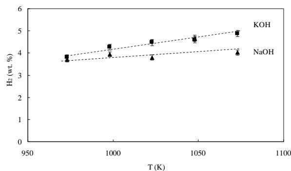
**Figure 2.** Evolution of H<sub>2</sub> storage capacity with the activation temperature,  $T$  (▲ NaOH, ■ KOH).
