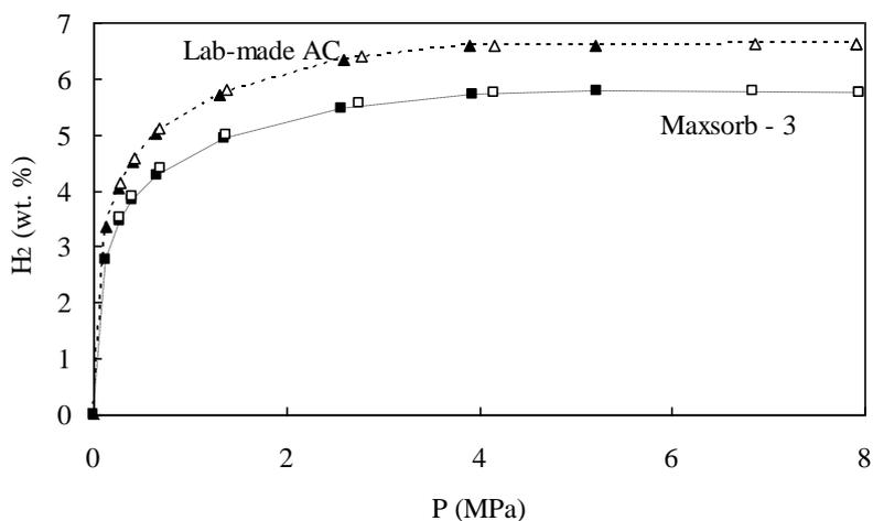
**Figure 5.** Total H<sub>2</sub> storage (wt. %) isotherms at 77K for Mawsorb-3 and for our best lab-made AC. Adsorption (full symbols) - desorption (open symbols).
