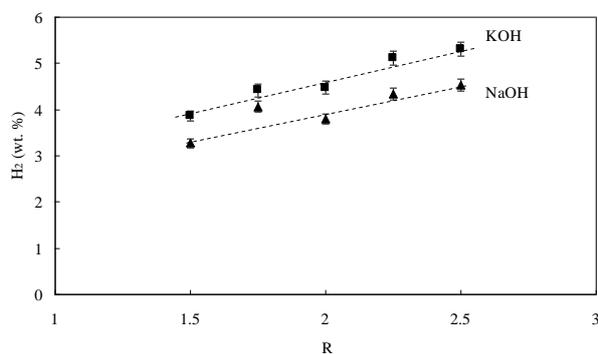
**Figure 1.** Evolution of H<sub>2</sub> storage capacity with the activation ratio,  $R$  (▲ NaOH, ■ KOH).
