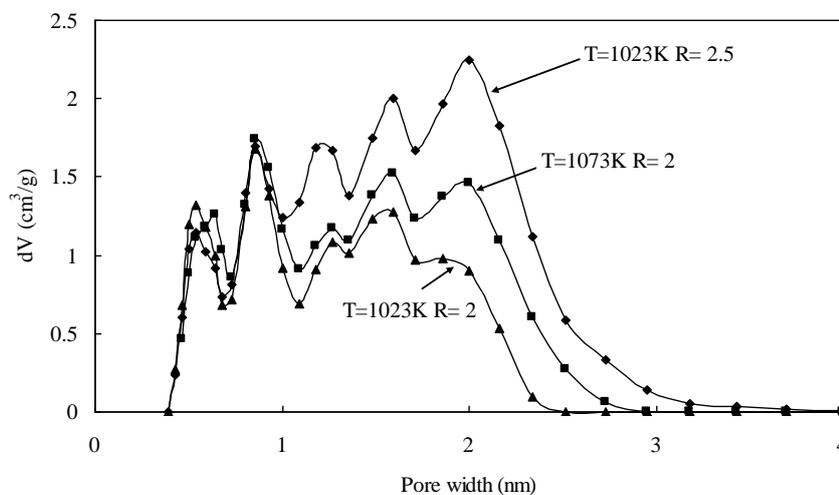
**Figure 3.** PSDs of three ACs prepared by KOH activation (▲  $T=1023$ K and  $R=2$ , ■  $T=1073$ K and  $R=2$  and ◆  $T=1023$ K and  $R=2.5$ ).
