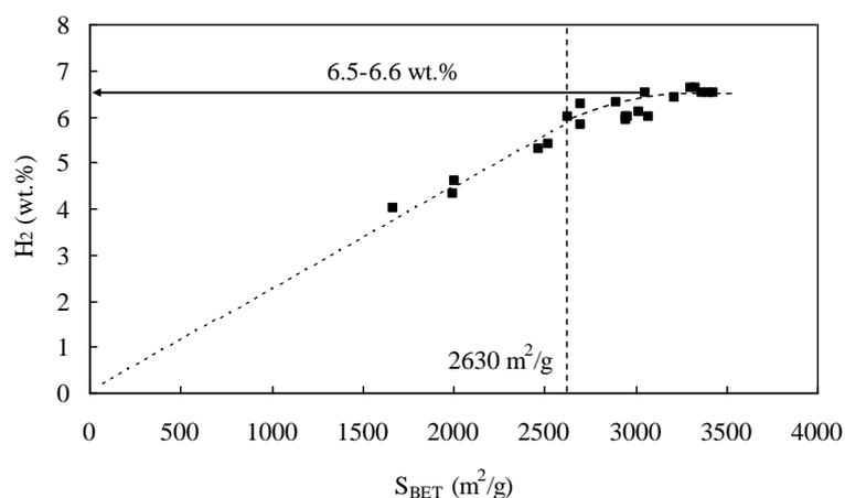
**Figure 4.** Total H<sub>2</sub> storage capacity (wt. %) as a function of  $S_{BET}$ .
