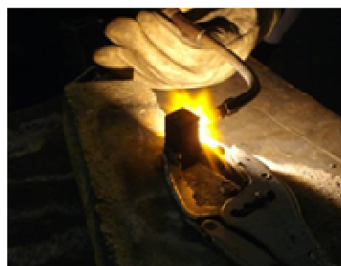
Figure 8. Carbon foam submitted to a 3000^\circ\text{C} oxyacetylenic flame in air. Neither flame nor smokes are emitted.
