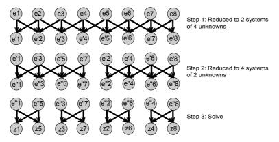
Figure 8: Modified Parallel Cyclic Reduction for n = 8: Communication pattern showing the dataflow and permutation of equations. Letters e' and e'' stand for updated equation.
