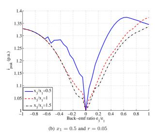
Fig. 7. Maximum peak current  $i_{peak}$  according to  $e_3/e_1$
