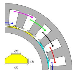
Fig. 8. Electromagnetic circuit and magnet shape parameters
