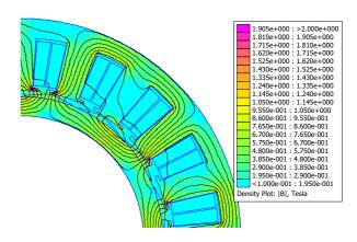
Fig. 10. Flux density at the maximum power point (FEA, [26])
