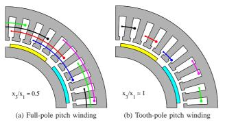
Fig. 4. Winding distribution effect on the inductance ratio
