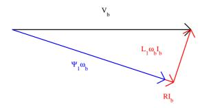
Fig. 1. Voltage vectorial diagram for the base point
