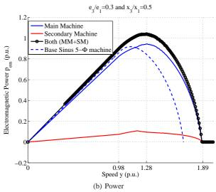
Fig. 2. Electromagnetic torque and power versus speed characteristics ( $x_1=0.28$  and r=0.08)
