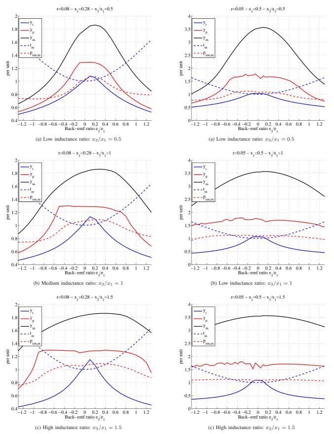
Fig. 5. Particular speeds, maximum torque and maximum em power change with  $e_3/e_1$  for machine with  $x_1=0.28$  and r=0.08
