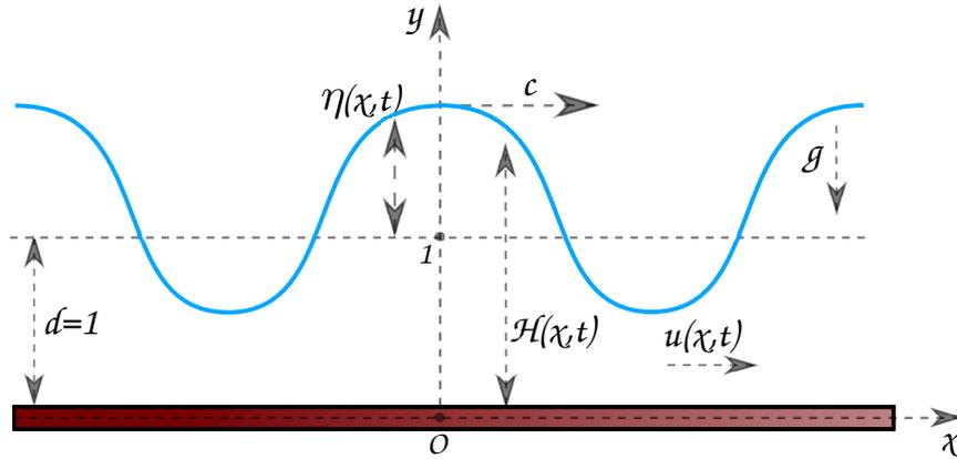
Figure 1. The sketch of the physical fluid domain.
