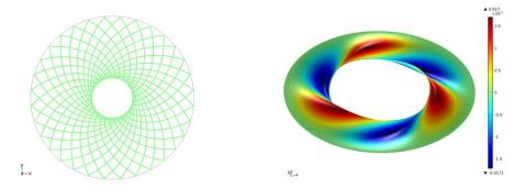
Figure 6. Buckling example with logarithmic spirals arrangement of fibers in the case of radial displacement ( $\tilde{u}_0 = 0.06$ ) and rotation (30 degrees) of the inner circle: Fiber pattern in the reference configuration (left); the shear strain relative to the initial fiber directions (right).
