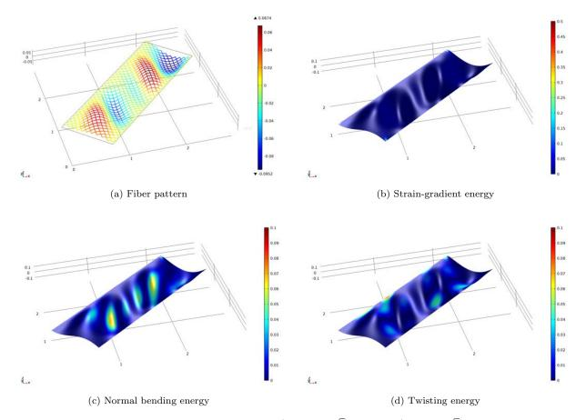
Figure 2. Case of initially straight fibers with compression ( $\tilde{v}_0 = 0.007\sqrt{2}$ ) and shear ( $\tilde{u}_0 = 0.05\sqrt{2}$ ) displacement imposed. on the derivatives of the displacement lying on the plane of the pantographic sheet and, in particular we impose:
