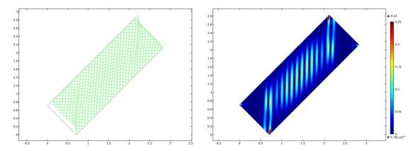
Figure 1. Geodesic buckling for the case of plane shear: fiber pattern (left) and the strain-gradient energy (right).
