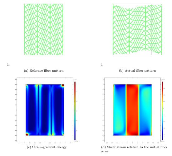
Figure 8. Bias extension test - displacement  $\tilde{u}_0 = 0.2$
