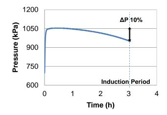
Figure 1 : Illustration of pressure variation during the oxidation of n-decane at 140°C, Induction Period (IP) equals 3.05 hours
