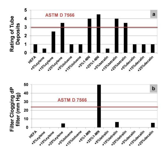
Figure 7 : Evaluation of thermal stability by JFTOT tests at 325°C (ASTM D3204) of HEFA-SPK, HEFA-SPK/cyclic molecules blends at 5-25%vol. a)Tube deposit rating after JFTOT test. b) Filter clogging measurement by pressure gradient variation after JFTOT test.
