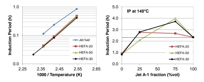
Figure 3: Induction period of a. HEFA-SPK and Jet fuel from 120-150°C, b. blends of HEFA-SPK/Jet A1 at 140°C
