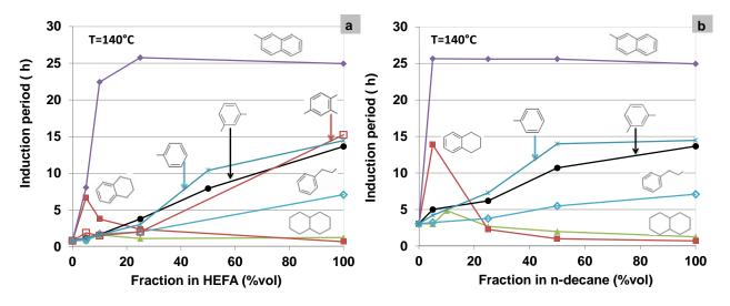
Figure 6 : Impact of the addition of cyclic compounds on the oxidation stability of: a) Cyclic compounds in HEFA-SPK at 140°C, b) Cyclic compounds in n-decane at 140°C. Symbols: full diamonds ♦ : 1 methylnaphthalene, full circles ●: xylene, star \*: toluene, blank squares I: 1,2,4, trimethylbenzene, blank diamonds ◊: n-PB, full squares I: tetralin, full triangles ▲ : decalin.
