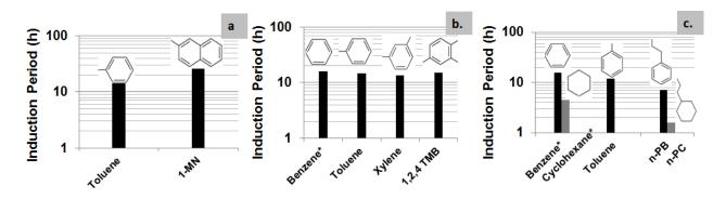
Figure 5: Effect of molecule structure on Induction Period at 140°C. a) Influence of number of benzene cycles. b) Influence of the number of branching on benzene ring. c) Influence of side chain length and hydrogenation.
