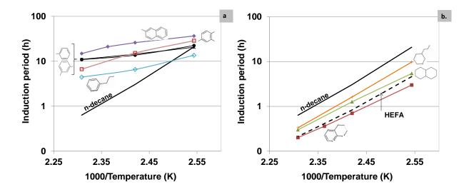
Figure 4 : Induction period of pure reagents, HEFA-SPK and n-decane function of inverse temperature from 120-160°C. a)alkylaromatics, b) naphthenes and tetralin. Symbols: full diamonds ◆ : 1-MN,full circles •: xylene, star \*: toluene (almost identical to xylene), blank diamonds ◊: n-PB, full squares ■: tetralin, full triangles ▲ : decalin, cross +: n-PC, bold solid line: n-decane andbold broken line: HEFA-SPK-
