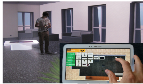
Figure 5: A combination of a CAVE and a tablet with D3PART.
