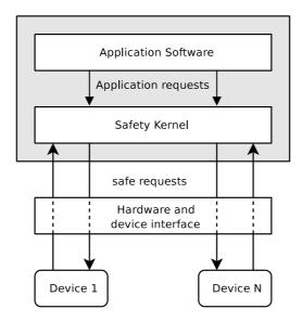
Figure 6: Magnetic Stereotaxis System's Safety Kernel (from [28])
