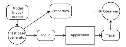
Figure 5: Test-case generator and trace verification framework (from [18])
