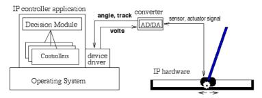
Figure 15: Inverted Pendulum (IP) device (from [27])
