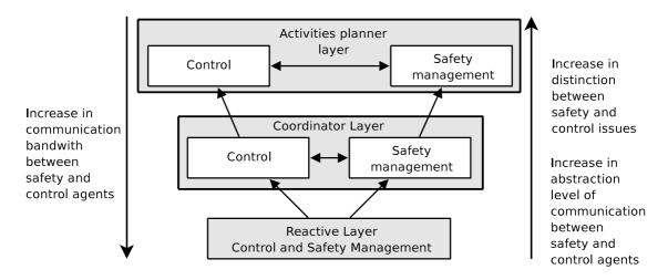
Figure 12: Safety component distribution in a three-layer architecture (from [25])
