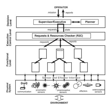
Figure 2: LAAS architecture for robot control
