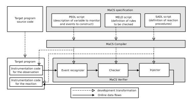
Figure 14: Monitoring Checking and Steering (MaCS) framework (derived from [27])
