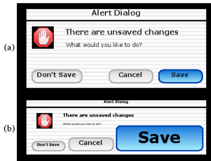
Figure XIV. Semantic Pointing: (a) a dialogue box in the visual space, (b) the same box in the motor space with semantic pointing – extracted of [18].
