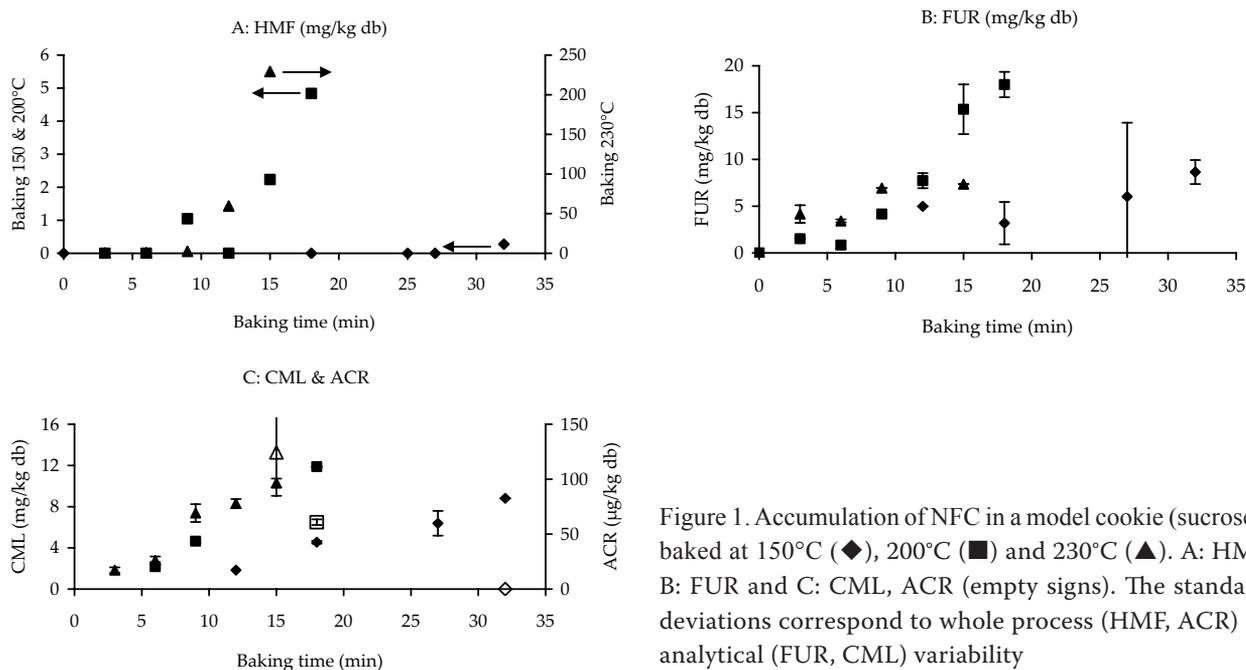
Figure 1. Accumulation of NFC in a model cookie (sucrose), baked at 150°C (◆), 200°C (■) and 230°C (▲). A: HMF B: FUR and C: CML, ACR (empty signs). The standard deviations correspond to whole process (HMF, ACR) or analytical (FUR, CML) variability
