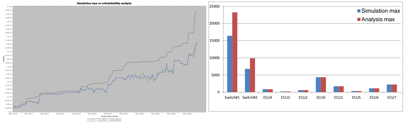
Figure 7: Case-study #1 – Left: upper bounds on WCTTs derived by schedulability analysis (black curve) and the maximum response times observed in simulation. The blue curve is obtained with null offsets for the nodes (i.e., zero-offset configuration), the green curve with random offsets. On average, the simulation with zero offsets leads to response times that are 21% less than the WCTTs, up to 48% maximum (with 5 points above 35%). Right: memory use in switches and nodes (in bytes) as derived by a long simulation (random startup offsets) and schedulability analysis.
