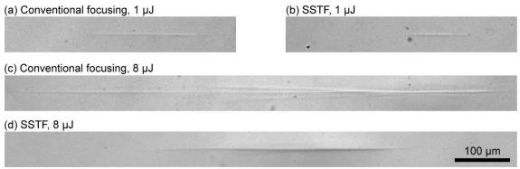
Figure 5. Microscope images of fs-laser-induced modifications within the bulk of a gelatine sample induced by conventional (a, c) focusing and SSTF (b, d) for 1  $\mu$ J (a, b) and 8  $\mu$ J (c, d) pulses, respectively.
