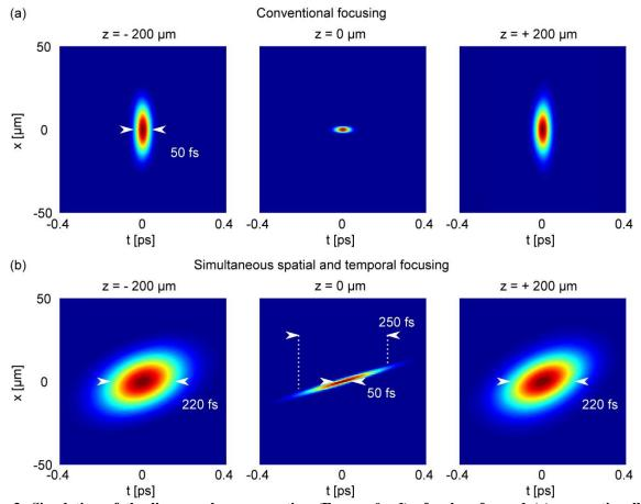
Figure 3. Simulation of the linear pulse propagation ( $E_{pulse} \approx 0~\mu J$ ) of pulses focused (a) conventionally and (b) using SSTF, showing x/t-intensity profiles nearby the focal plane ( $z = -200~\mu m$ , 0  $\mu m$ , + 200  $\mu m$ ).
