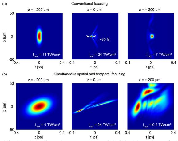
Figure 4. Simulation of the nonlinear pulse propagation ( $E_{pulse} \approx 4~\mu J$ ) of pulses focused (a) conventionally and (b) using SSTF, showing x/t-intensity profiles nearby the focal plane ( $z = -200~\mu m$ , 0  $\mu m$ , + 200  $\mu m$ ).
