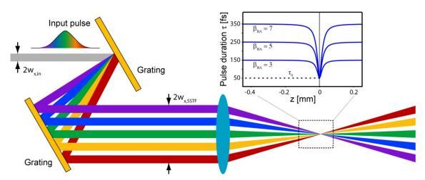
Figure 2. Scheme of simultaneous spatial and temporal focusing based on a single pass parallel grating compressor configuration. The inset illustrates the development of the pulse duration around the focal region depending on the spatial chirp beam aspect ratio  $\beta_{BA}$ .
