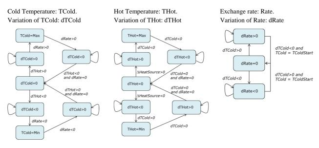
Note:  $\Delta$ HeatSource>0 (resp. < 0) means an increasing (resp. decreasing) of heat source. Thus we finally obtain a set of paths containing all potential behaviors. The following picture describes one of them.
