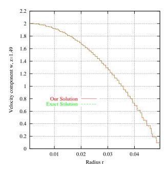
FIG. 16 – Velocity profile near the outlet
