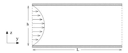
FIG. 4 – Geometry, Poiseuille flow between two parallel planes
