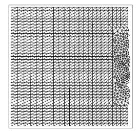
Figure 13: Mesh at the inlet
