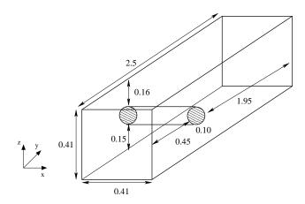
Figure 12: Geometry, 3D flow past a cylinder
