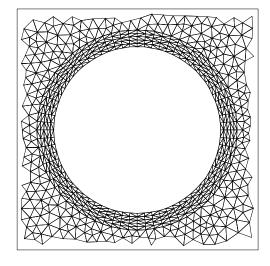
Figure 14: Mesh around the cylinder
