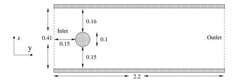
FIG. 11 - Geometry, 2D flow around a disc
