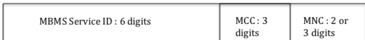
Figure 32 Structure of TMGI
