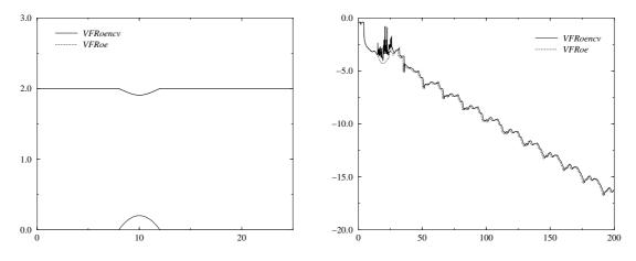
Figure 27: Subcritical flow : water height
