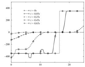
Figure 17: Vacuum occurence over a step : water height
