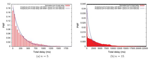
Fig. 6. Analytical total delay PMFs for M/M/1 and M/G/1 queues vs. simulations.
