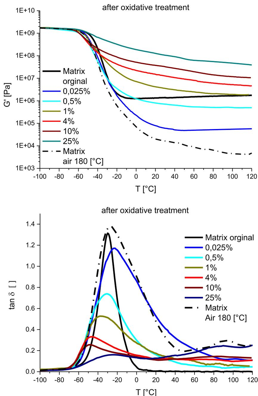
**Fig. 11.** Effect of nanofiller content on the thermo-mechanical properties of the epoxy-Sn2 nanocomposites which underwent oxidation treatment: Shear storage modulus  $G'$  (top) and loss factor  $\tan(\delta)$  (bottom) as function of temperature: nanofiller content is in the range of 0.025–25 mol% amino protons.
