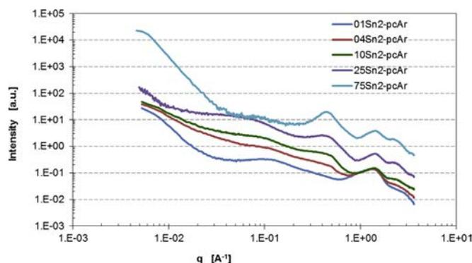
**Fig. 7.** SAXS scattering patterns of epoxy nanocomposites with different contents of Sn2, ranging from 1 mol% to 75 mol%, corresponding to 2–76 wt%, which were additionally post-cured under argon (12 h at 180 °C).
