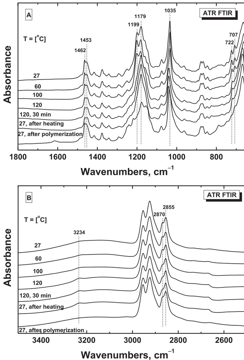
**Fig. 2.** ATR FTIR spectra of a neat Sn2 cage sample heated to 27, 60, 100, 120 (repeated measurement after 30 min), and thereafter cooled back to 27 °C. A spectrum of a sample rapidly polymerized at 240 °C is shown for comparison. Top: range of sulfonate groups stretching vibrations and of aliphatic C–H bending and twisting; Bottom: range of O–H and N–H stretching.
