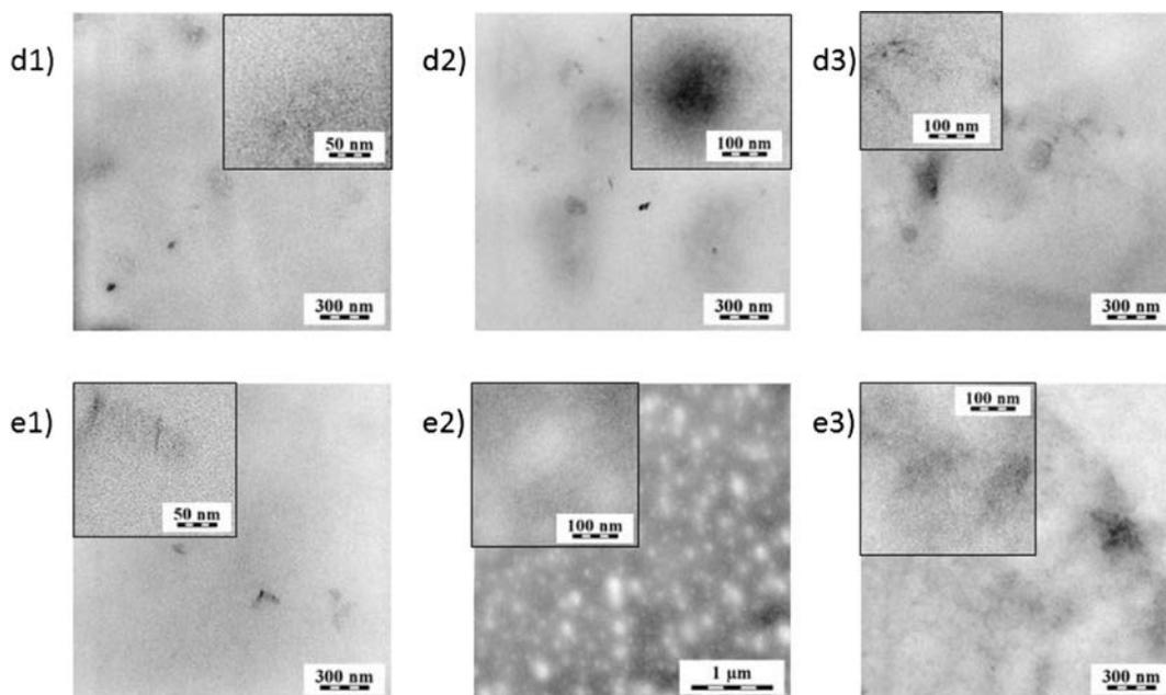
**Fig. 4.** Transmission electron microscopy images of Sn2 nanocomposites with DGEBA-D2000: with 25 mol% Sn2 (d1–d3), and 50 mol% Sn2 (e1–e3), which underwent normal cure (d1, e1), additional 12 h post-cure under argon (d2, e2), or additional 12 h oxidation treatment (d2, e2).
