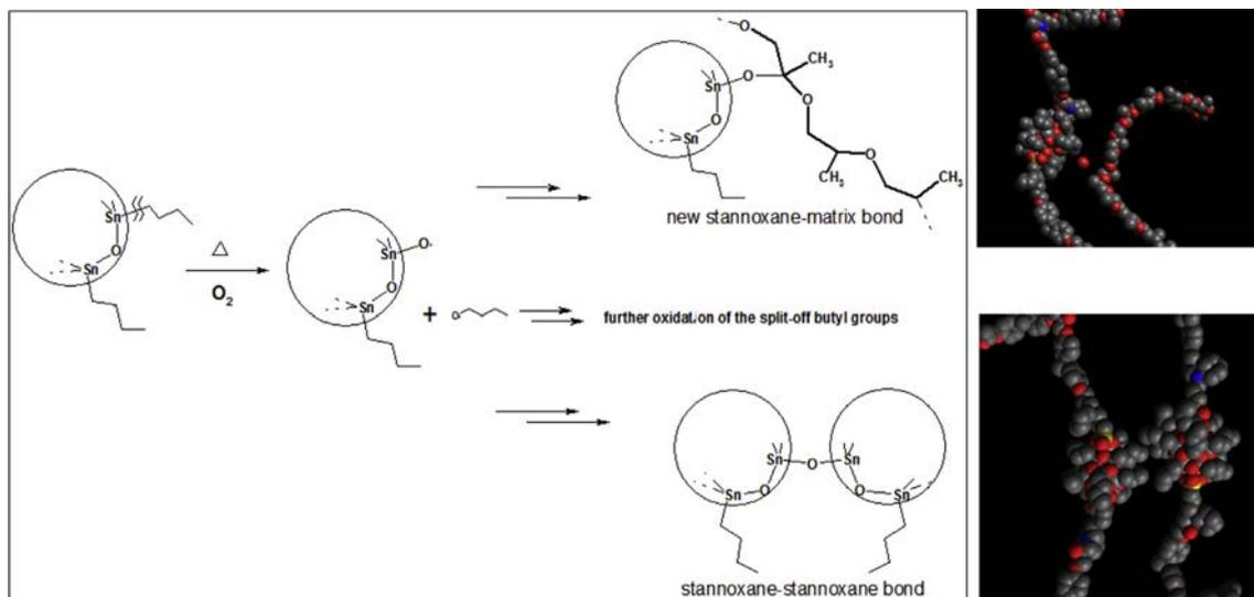
**Scheme 8.** Oxidative crosslinking reactions of the stannoxane nano-building blocks with the matrix and with each other, as proven by  $^1\text{H}$  NMR experiments in Ref. [40].
