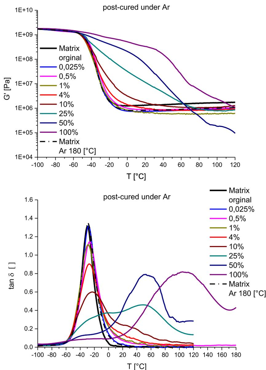
**Fig. 10.** Effect of nanofiller content on the thermo-mechanical properties of the epoxy-Sn2 nanocomposites which underwent post-cure under argon (nanofiller polymerization): Shear storage modulus  $G'$  (top) and loss factor  $\tan(\delta)$  (bottom) as function of temperature: nanofiller content is in the range of 0.025–100 mol% amino protons.
