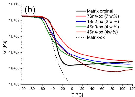
**Fig. 13.** Comparison of the anti-oxidative effect of Sn2 cages in the DGEBA-D2000 matrix with the effect of previously studied [40] Sn4 and Sn0, the latter of which was further studied in a work which is being prepared for publication;  $G = f(T)$  at (a) high filler concentrations around 20 wt%; (b) at low filler concentrations.
