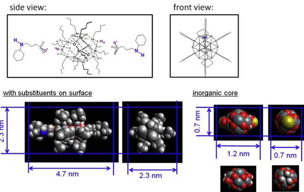
**Scheme 1.** Ellipsoid butylstannoxane dodecamer nano-building block used in this work:  $[(n\text{C}_4\text{H}_9\text{-Sn})_{12}(\text{O})_{14}(\text{OH})_6][\text{O}_3\text{S}-(\text{CH}_2)_3\text{-NH-C}_6\text{H}_{11}]_2$ .
