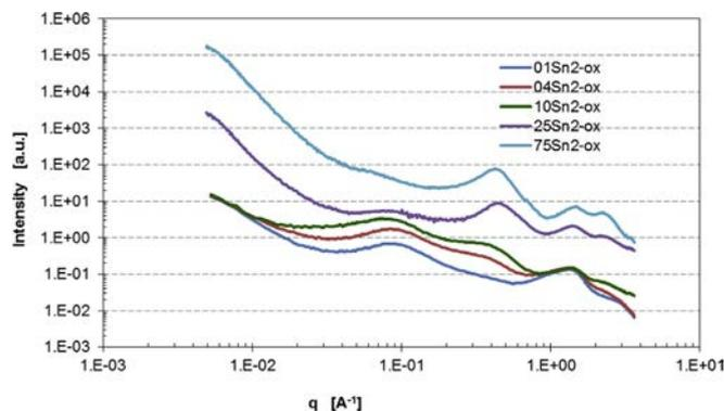
**Fig. 8.** SAXS scattering patterns of epoxy nanocomposites with different contents of Sn2, ranging from 1 mol% to 75 mol%, corresponding to 2–76 wt%, which additionally received oxidation treatment (12 h in circulating air at 180 °C).
