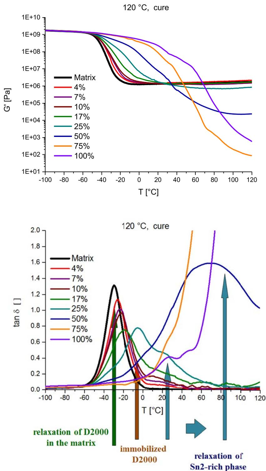
**Fig. 9.** Effect of nanofiller content on the thermo-mechanical properties of normally cured epoxy-Sn2 nanocomposites: Shear storage modulus  $G'$  (top) and loss factor  $\tan(\delta)$  (bottom, with assignment) as function of temperature: nanofiller content is in the range of 4–100 mol% amino protons.
