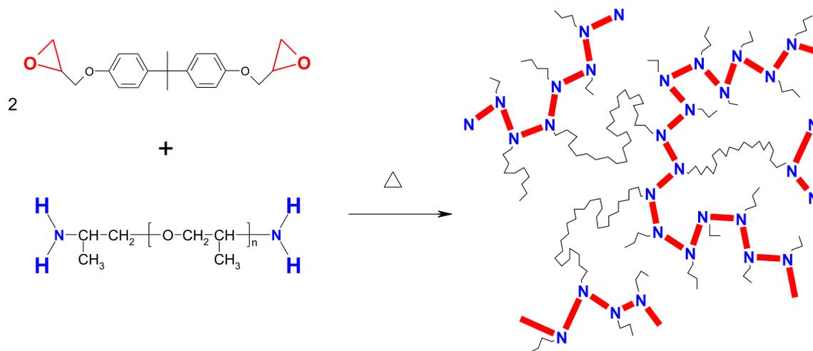
**Scheme 4.** Synthesis of the polymer matrix from diglycidylether of bisphenol A (DGEBA) and poly(oxypropylene)  $\alpha,\omega$ -diamine “Jeffamine D2000” (34-mer). In the matrix structure, DGEBA forms the more rigid chains (red, bold lines) which are interconnected by long elastic chains of D2000 (black thin lines) at the end of each DGEBA repeat unit. (For interpretation of the references to colour in this figure legend, the reader is referred to the web version of this article.)
