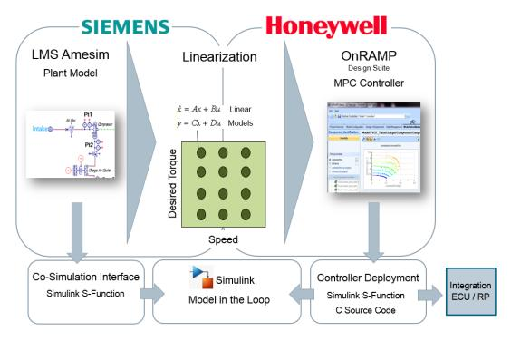
The first step of the process is to identify inputs, outputs, disturbances and scheduling variables to the controller. This is determined thanks to a modeling convention in LMS Amesim. In practice, the interface between the two tools is concretized by an interface block included in the plant model which defines the actual control I/O.
