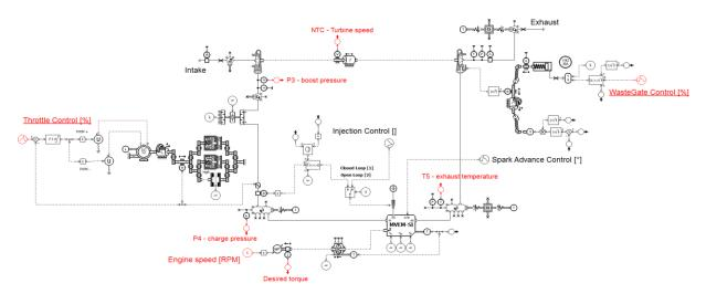
The control problem is expressed here in terms of tracked control inputs (sensor signals) – boost and charge pressure, outputs (actuator commands) – throttle and waste gate and constraints – turbocharger speed and exhaust temperature. The controller is evaluated by applying a given engine speed and boost and charge pressure setpoints and analyzing the results in terms of charging pressure and torque production.
