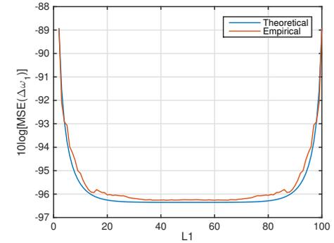
Fig. 7. Theoretical and empirical MSEs for 2-D ESPRIT (fast SVD) versus  $L_1$ , ( $L_2 = 4$ ).  $(\alpha_a, \omega_a) = (-0.1, 0.2\pi)$ ,  $(\alpha_b, \omega_b) = (-0.1, 0.4\pi)$ ,  $(M_1, M_2) = (100, 100)$ , SNR = 40 dB.
