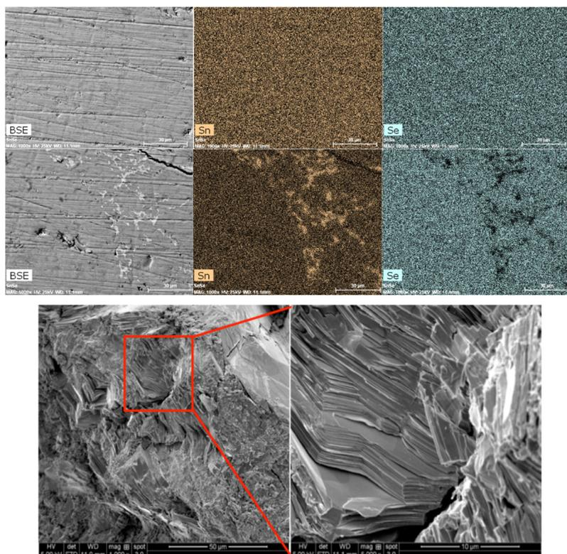
FIG. 2. (Top panels) X-ray mappings indicating a good chemical homogeneity of the samples. (Middle panels) X-ray mappings highlighting the small fraction of elemental Sn present in the samples. The scale bar stands for  $30 \mu\text{m}$  in all images. (Bottom panels) SEM fracture images of SnSe after SPS treatment.
