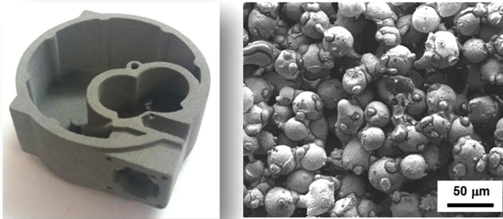
Figure 2. Left: picture of a porous preform made by SLS containing Al–Cu–Fe–B QC particles and a polymer binder. The lateral dimension of the preform is 5 cm. Right: SEM image of the mixed powder after selective sintering showing the formation of polymer bridges connecting the QC particles.
