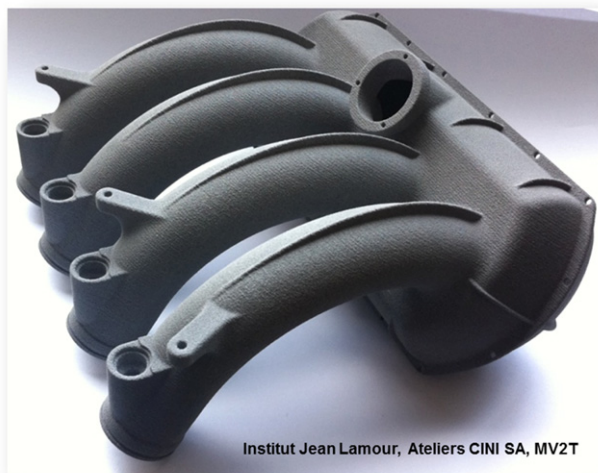
Figure 4. Picture of an intake manifold made of a polyamide composite reinforced by QC particles. This part is used in automotive industry and is produced by SLS in a single processing step. The size of the component is about 20×30×40 cm. Reproduced from [14], Copyright (2012), with permission from Elsevier.
