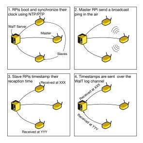
Figure 4. Clock drift measurement scenario
