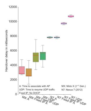
Figure 8. Measured Wi-Fi handover delay
