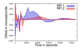
Figure 5. NTP offset variation between two nodes and the time master
