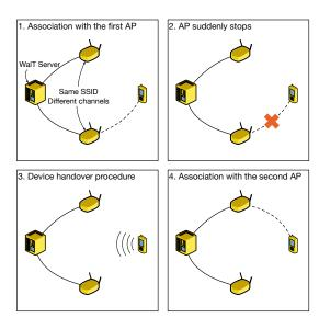
Figure 7. Wi-Fi handover measurement scenario
