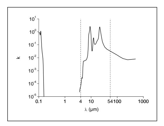
Figure 3: extinction index spectrum of  $a-SiO_2$  (taken from [9]).
