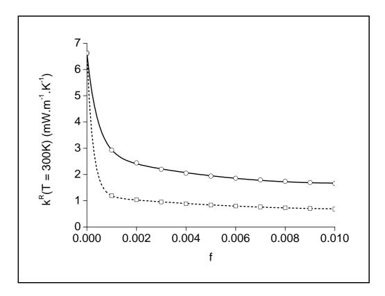
**Figure 10:** dependence of the radiation thermal conductivity  $k^{R}(T)$  of a NSM (at T = 300K) as a function of the microparticle population volume fraction  $f^{\mu p}$ . The circles and the solid curve refer to a NSM made of a a-SiO<sub>2</sub> nanoparticle population ( $d^{np} = 10$  nm and  $f^{np} = 10\%$ ) and of a a-SiO<sub>2</sub> microparticle population ( $d^{\mu p} = 1 \mu m$ ). The squares and the dashed curve
