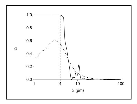
**Figure 8:** effective albedo  $\Omega_{\lambda}^{e}$  spectra (i) of the a-SiO<sub>2</sub> microparticle population ( $d^{\mu p} = 1 \ \mu m$ and  $f^{\mu p} = 1\%$ ) (solid line), and (ii) of the graphite microparticle population (same  $d^{\mu p}$  and  $f^{\mu p}$ ) (dashed line).
