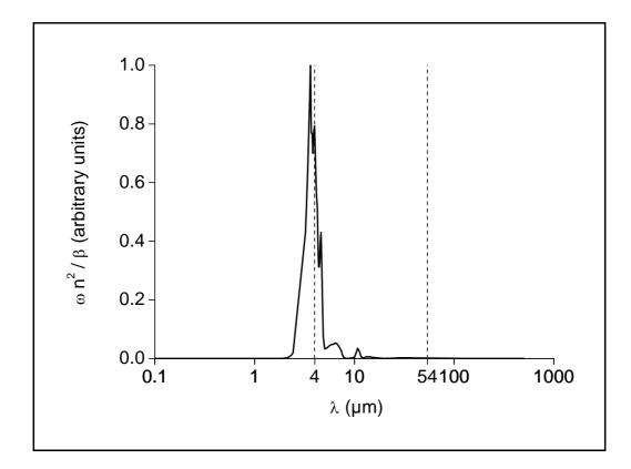
Figure 4: calculated  $\omega_T(\lambda) n_{\lambda}^2 / \beta_{\lambda}^e$  spectrum of the nanoporous a-SiO<sub>2</sub> matrix at room temperature.
