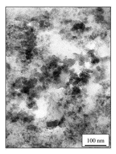
Figure 2: TEM image of the nanoporous a-SiO<sub>2</sub> matrix appearing in figure 1.
