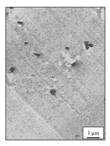
**Figure 1:** TEM image of a particular NSM made of a nanoporous  $a-SiO_2$  matrix and of crystalline SiC microparticles. The nanoporous matrix appears as the gray phase, whereas the SiC microparticles are the dark inclusions. The white zones as well as the parallel scratches apparent on this image are due to polishing imperfections.
