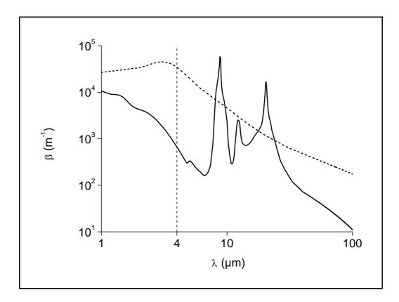
**Figure 9:** effective extinction coefficient  $\beta_{\lambda}^{e}$  spectra (i) of the a-SiO<sub>2</sub> microparticle population ( $d^{\mu p} = 1 \ \mu m$  and  $f^{\mu p} = 1\%$ ) (solid line), and (ii) of the graphite microparticle population (same  $d^{\mu p}$  and  $f^{\mu p}$ ) (dashed line).
