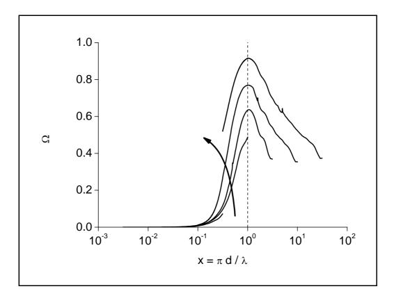
**Figure 11:** effective albedo  $\Omega_{\lambda}^{e^{-\mu p}}$  spectra of 5 graphite microparticle populations of identical volume fractions ( $f^{\mu p} = 1\%$ ) differing only by the microparticle uniform diameter  $d^{\mu p}$  (100 nm, 300 nm, 1 µm, 3 µm and 10 µm). The 5  $\Omega_{\lambda}^{e^{-\mu p}}$  spectra are plotted *versus* the size parameters  $x_{\lambda}^{\mu p} = \pi d^{\mu p} / \lambda$ . The arrow on the figure indicates increasing values of  $d^{\mu p}$ .
