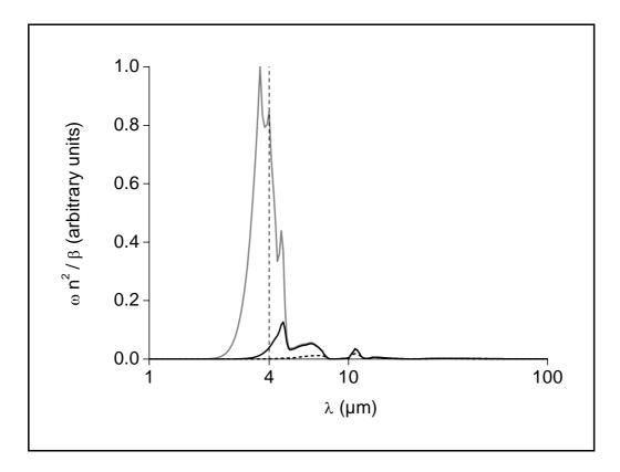
**Figure 6:** calculated  $\omega_T(\lambda) n_{\lambda}^2 / \beta_{\lambda}^e$  spectra (at room temperature) (i) of the NSM containing a a-SiO<sub>2</sub> microparticle population (solid line), and (ii) of the NSM containing a graphite microparticle population (dashed line). The grey solid line represents the  $\omega_T(\lambda) n_{\lambda}^2 / \beta_{\lambda}^e$  spectrum of the nanoporous a-SiO<sub>2</sub> matrix (previously exhibited in figure 4).
