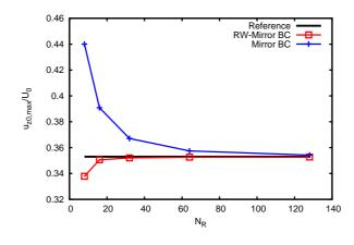
Figure 13: Maximum axis velocity for Rayleigh Benard convection
