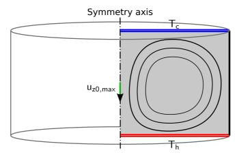
Figure 12: Simulated system for the Rayleigh Benard convection
