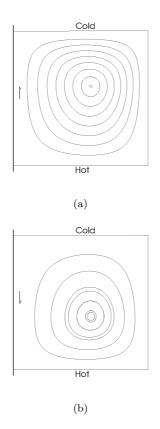
Figure 14: Velocity streamlines for Rayleigh-Benard convection:14(a) initial cold temperature, 14(b) initial hot temperature
