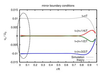
Figure 9: Typical solution for the wormersley flow with  $\alpha = 20$ . Mirror boundary conditions  $(N_R = 32)$
