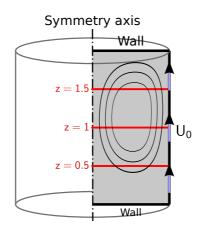
Figure 15: Simulated system for the side driven cavity
