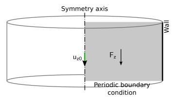
Figure 6: Simulation domain of the Poiseuille Hagen flow
