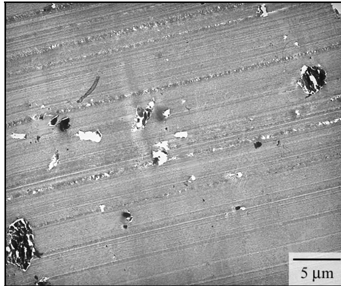
Figure 1: TEM image at a micrometric scale of a particular NSM made of a nanoporous a-SiO 2 matrix and of crystalline SiC microparticles. The nanoporous matrix appears as the grey phase, whereas the SiC microparticles are the dark inclusions. The white zones, corresponding to holes, as well as the parallel scratches apparent on this image are due to sample preparation.
