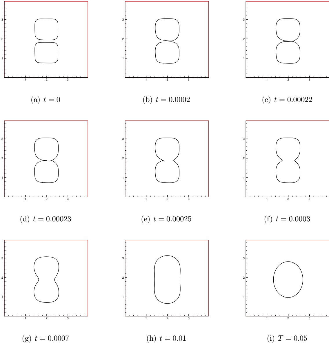
FIGURE 5.5. Topology changes. Two square-like shapes merge under the level set evolution of Willmore flow.
