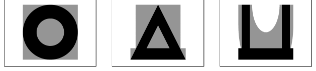
Figure 2: The silhouettes from Figure 1 are geometrically consistent (relative to three orthogonal orthographic projections), since each silhouette is contained in the reprojection (in gray) of the intersected visual cones associated to the other views. See Proposition 1.
