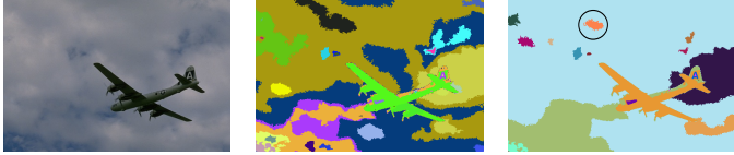
Figure 4: Illustration of causality principle violation. Left: input image; Middle and right: randomly colored simplified image with \lambda_{s_1} = 100 and respectively \lambda_{s_2} = 500 . The orange shape on top middle of the right image (surrounded by a black circle) is preserved for \lambda_{s_2} = 500 , while it is removed for \lambda_{s_1} = 100 in the middle image.
