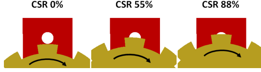
FIGURE 2. RELATIVE POSITIONS OF THE TOOTHED WHEEL AND SIREN NOZZLE FOR DIFFERENT CSR (0%, 55% AND 88%).
