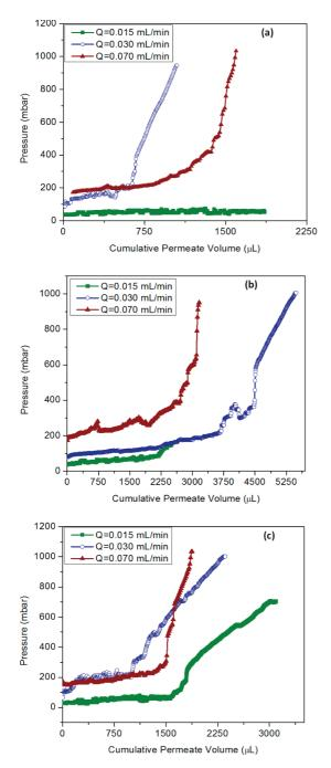
**Figure 2.** Pressure drop vs cumulative permeate volume at different flow rates (15, 30, and 70  $\mu$ L/min) for different solution ionic strengths: (a) 0.01, (b) 10, and (c) 100 mM.
