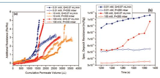
Figure 4. (a) Comparison of additional hydrodynamic resistances at low (0.01 mM), moderate (10 mM), and high (100 mM) ionic strengths. (b) Specific deposit resistances for low (0.01 mM) and high (100 mM) solution ionic strengths. The experiments are performed at constant pressure (200 mbar) and constant flow rate (70  $\mu$ L/min).
