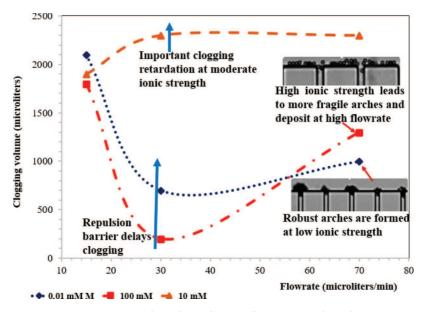
Figure 5. Filtered volume leading to clogging determined for different filtration flow rates and for different ionic strengths.
