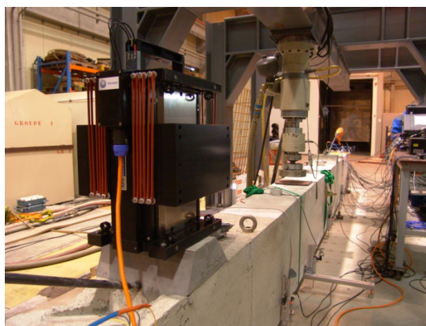
Figure 3: The specimen on the test bench with the shaker and the hydraulic jack.
