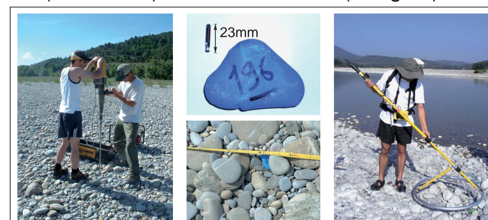
Fig.10 Setting up of scour chains and PIT tags at RK 205
