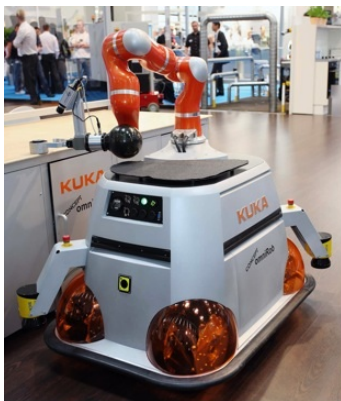
Figure 2: Example of a mobile manipulator: “concept omniRob” © at Automatica 2008 exhibition – KUKA Roboter GmbH
