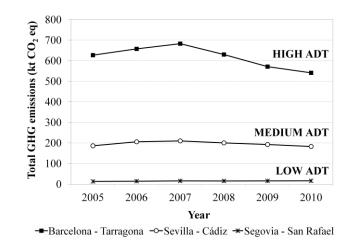
Figure 1. Evolution of total GHG emissions for three motorway stretches during 2005-2010 for average speeds of 120 km/h and 85 km/h for light and heavy vehicles
