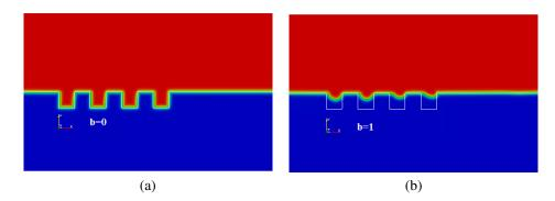
Figure 5: (a) and (b) illustrate respectively the cavities filling for  $L_{ref} = 0.1 \, mm$  with b = 0 and b = 1.
