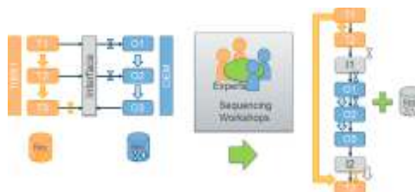
Fig. 6 : Effect of position in the sequence on the data flow between supplier and OEM runnables
