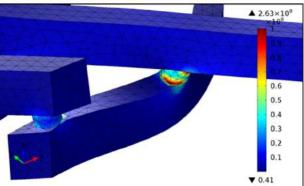
Fig. 2 Three-dimensional simulation for a pantographic structure as studied in Ref. [359]. Top: the deformation energy is stored in the pivots; bottom: the employed mesh is visible (original picture by the authors).
