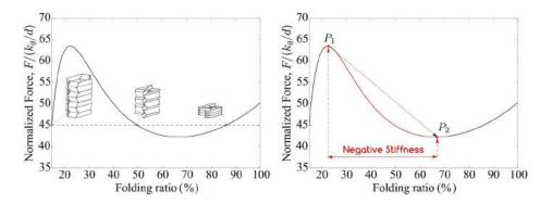
Fig. 6 Left: three different configurations of the papermade Tachi-Miura polyhedron (studied in Ref. [275]) under the same normalized force; right: force-folding ratio relationship and snap-through response (original rendering of pictures provided by the authors)
