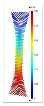
Fig. 16 Three-dimensional simulation for a pantographic structure in traction as studied in Ref. [359] (original picture by the authors)
