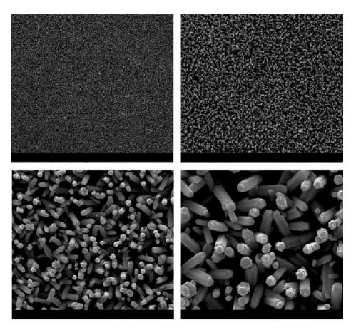
Fig. 12 ZnO nanoarray (respectively,  $300 \times$ ,  $1200 \times$ ,  $5000 \times$ , and  $10,000 \times$  from top left to bottom right) (Reproduced with permission from Ma et al. [298]. Copyright 2008 by Elsevier.)
