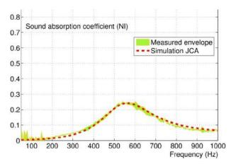
Fig. 8 Sound absorption coefficient at ambient condition of temperature and pressure for the system studied in Ref. [276] and represented in Fig. 7. Measurement is represented by the thick line and simulation by the dashed one (original picture by Professor Claude Boutin).
