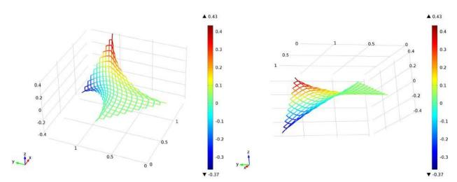
Fig. 19 Out-of-plane twisting of a squared pantographic sheet as studied in Ref. [358]. The picture is relative to a continuum simulation, and that the curves represent sets of material points which are straight lines in the reference configuration (original picture by the authors).
