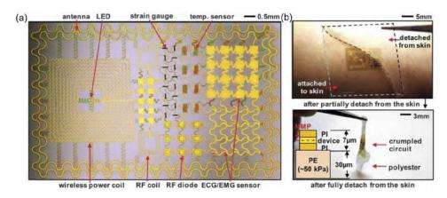
Fig. 20 Epidermal flexible plate (Reproduced with permission from Kim et al. [361]. Copyright 2011 by AAAS.)
