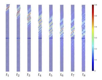
Fig. 18 Damping of a wave by means of an array of vertical springs in a pantographic structure (Reproduced with permission from Madeo et al. [240]. Copyright 2014 by Proceedings of the Estonian Academy of Sciences.)
