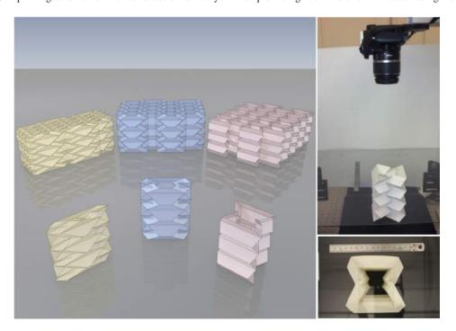
Fig. 5 Handicraft metamaterial exhibiting interesting mechanical properties (high damping, negative stiffness, snap-through, etc.): Tachi-Miura polyhedron realized by means of origami structures made of paper as studied in Ref. [275]. Left: digital image of the prototypes; right: photo of the top of the prototype (original pictures by the authors).
