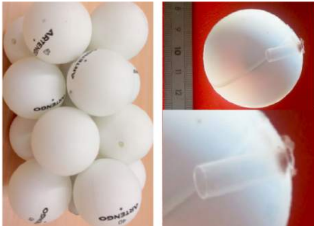
Fig. 7 Another example of handcraft metamaterial: hollow plastic spheres (138 mm high) with a central impervious cylinder studied in Ref. [276]. Spheres might be impervious hollow spheres, or resonators, or both (see Table 1 in the reference paper for details). The interspheres space might be occupied either by air or filled by a granular medium. Left: geometry of the prototype; middle: a prototype; right: cut of the two types of Helmholtz resonators (original pictures by Professor Claude Boutin).
