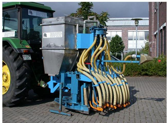
**Fig. 1** A tractor-attached experimental device for slurry application that comprises application parts from slurry tanks used in practice
