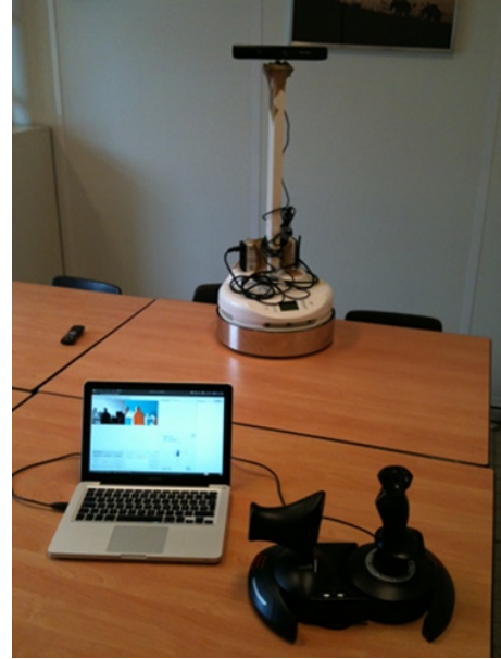
Figure 3: The Pekee II mobile robot in our setup with the Kinect module during the shooting of the dataset.
